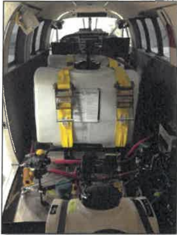
Figure 9: Spray system installed in the cabin area of King Air A90.
