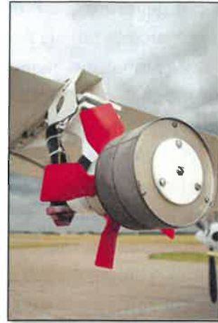
Figure 10: Micronair AU4000 device integrated on wing of King Air A90.
