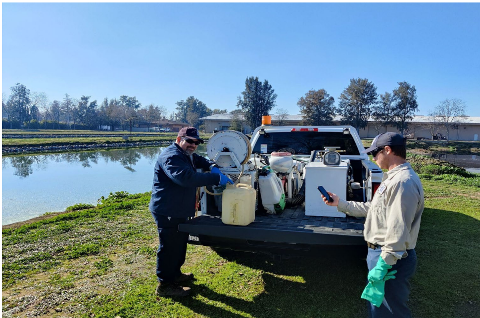
Field Technicians measuring spray output during truck equipment calibration
